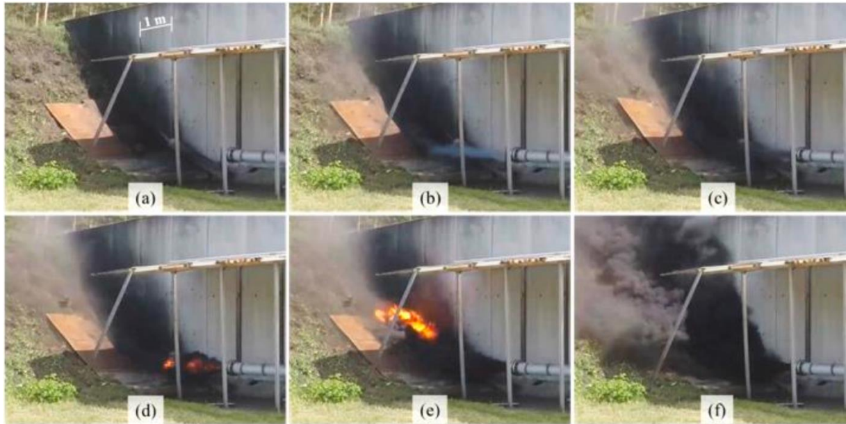
Figure 27 Series of images showing the venting of a TFE explosive decomposition with 10 bar TFE compressing 0.4 bar air.
