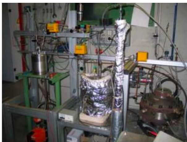
Figure 19 Experimental set up for the MIT determination of TFE and TFE mixtures
