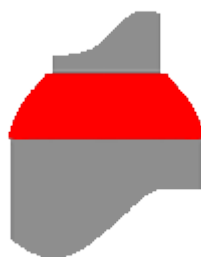
Figure 16 European colour-coding for flammable gases. Shoulder colour: red. Picture from [4]
