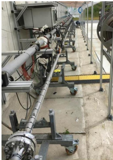
Figure 26 Industrial scale compression test apparatus during the installation of the 2.5-inch pipe without the thermal insulation present
