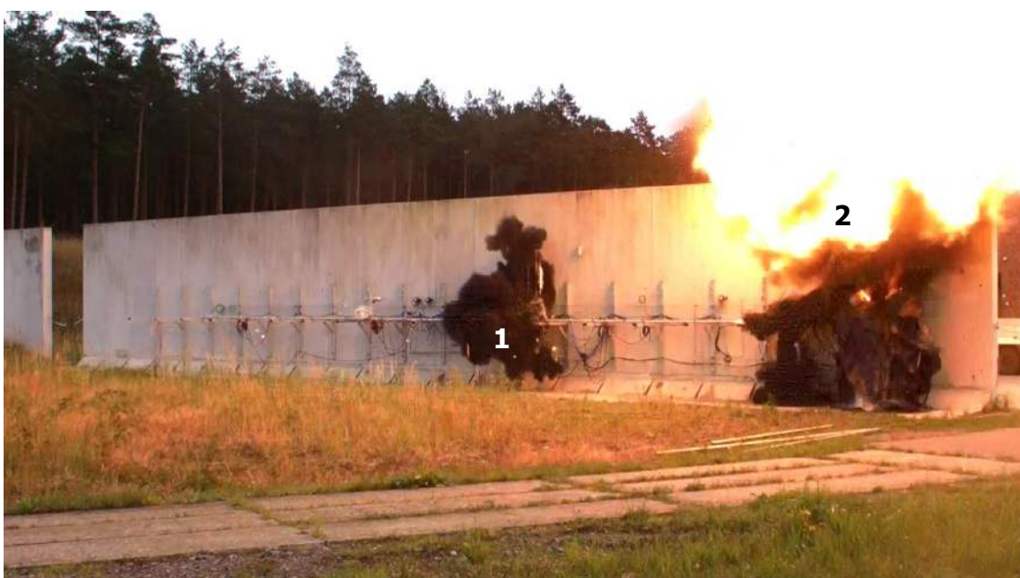
Figure 9 Picture taken during an ignition of TFE induced by adiabatic compression of air in a large-scale facility
