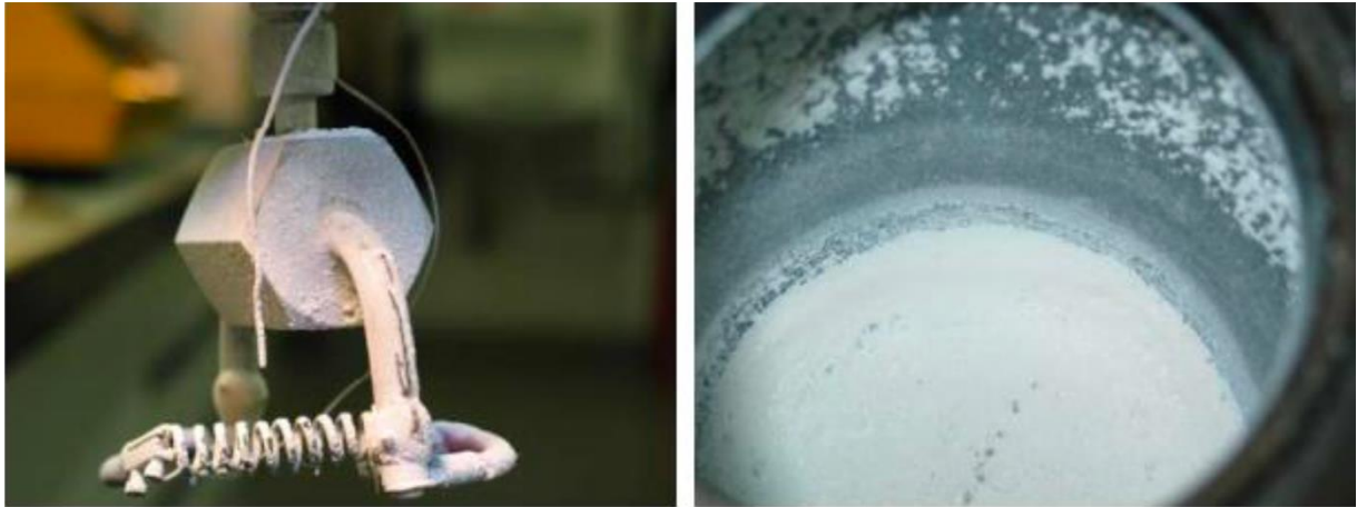
Figure 20 Formation of PTFE during the tests (left; with the spiral wire, right; 3-L autoclave after the tests with the naked heating cartridge)
